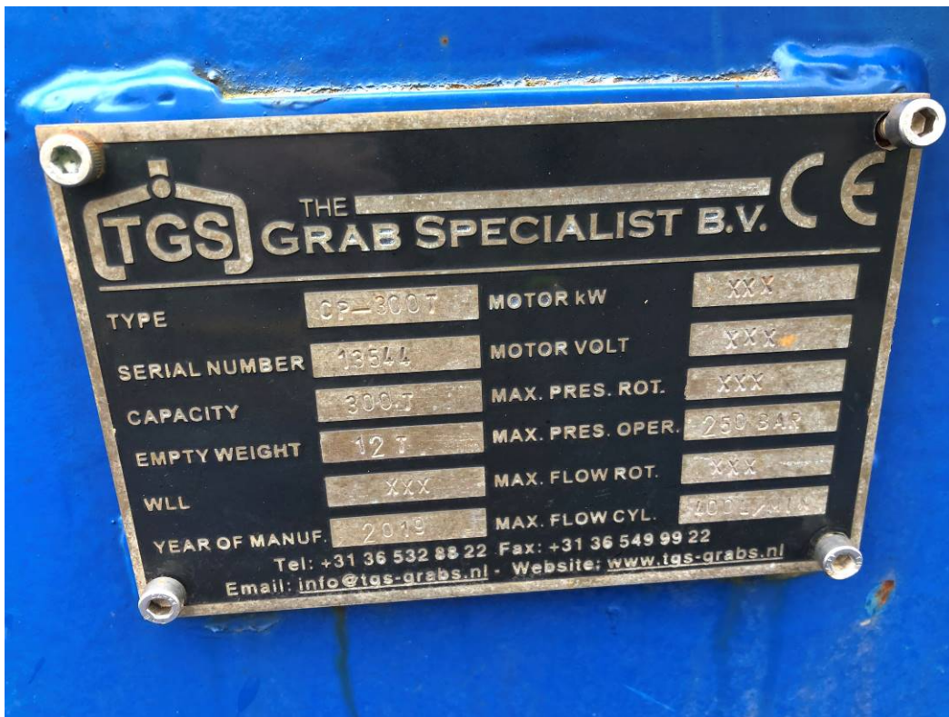
8. Name plate showing puller capacity of 300MT
