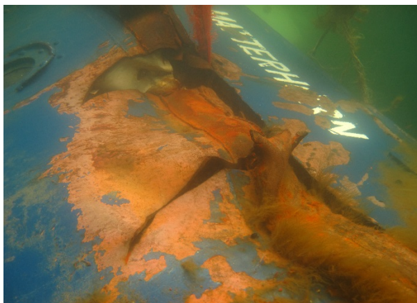
Shows hull damage on starboard side.
