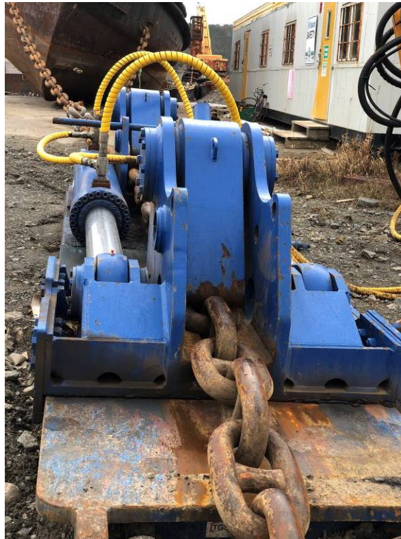
7. Chain puller used to haul vessels up the "slipway"
