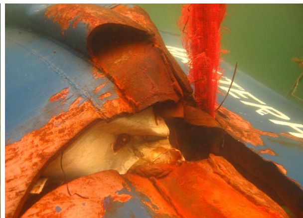
Shows hull damage on starboard side.
