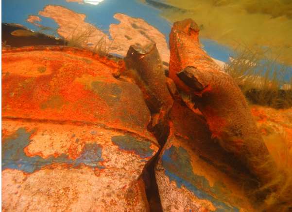
Shows hull damage on starboard side.
