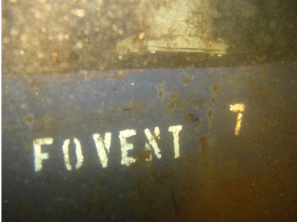
Shows F/O vent capped.
