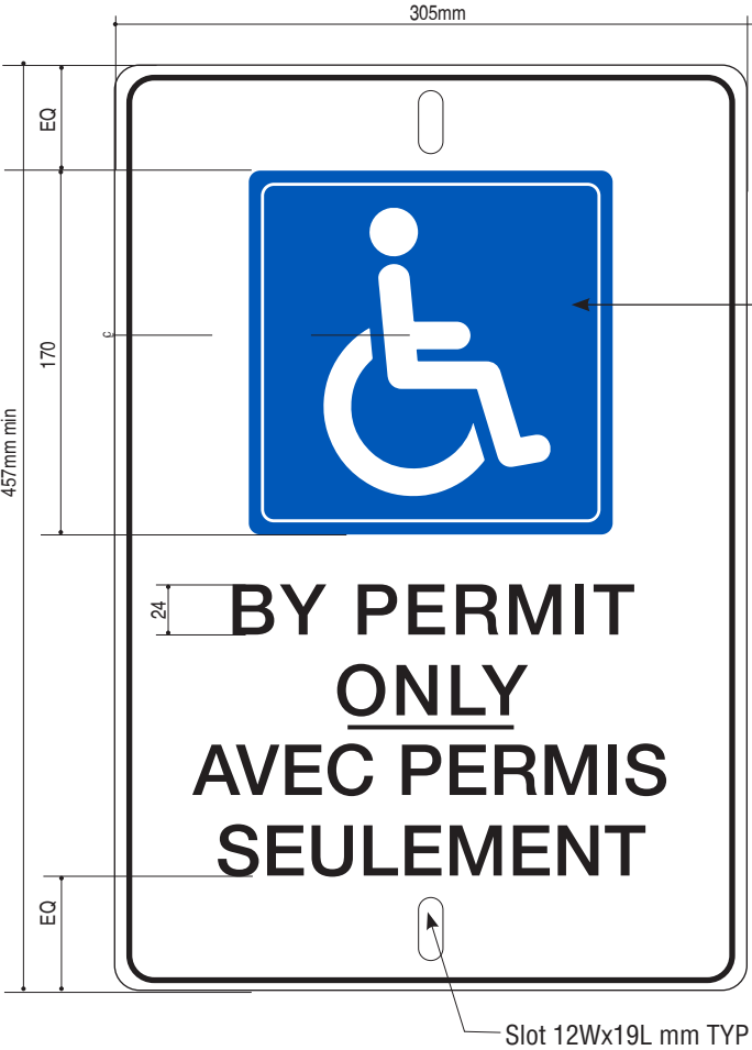
M11.2 Notification Sign - Parking and Traffic-By Permit Only 305mm x 457mm x 3mm Scale 1:4 3mm thick Aluminum with radius corners, with Digital print on reflective applied to face. Sign to be installed to existing surface using appropriate screws and fasteners, 1500 ± 25mm to floor from sign center, centered on parking stall.
