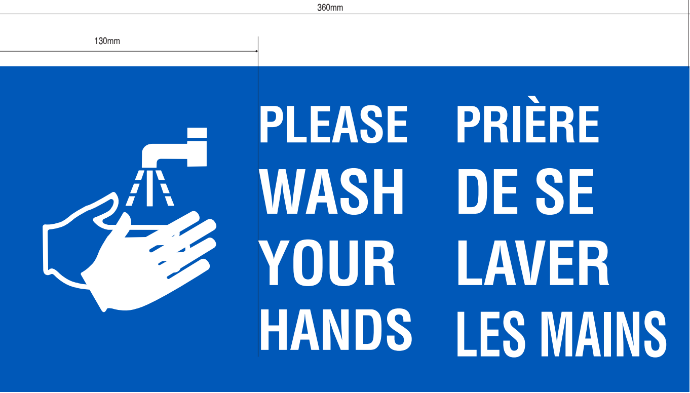
W7-W-325 Safety Sign - Please Wash Your Hands 360mm x 170mm x 3mm Scale 1:2 3mm ACM with direct surface printed graphics. Clear protective laminate. Mounted near the sink in all washrooms. Background colour: to match DARK LLUE (refer to page 3)
