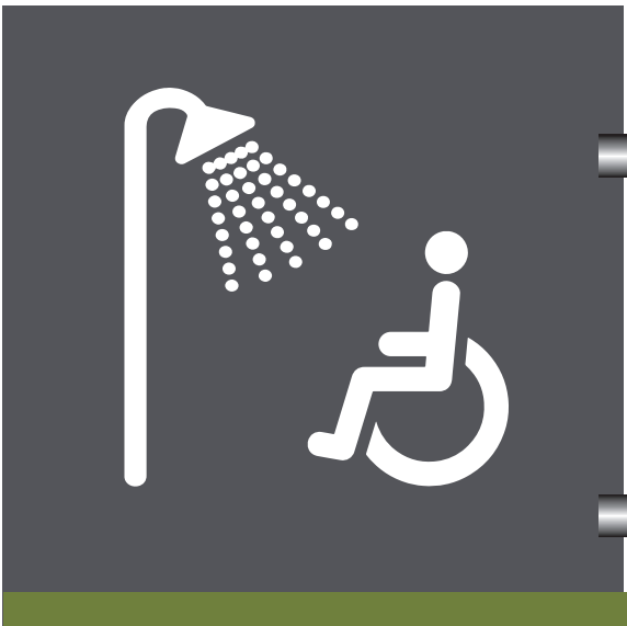
AS2.7-P-08a Amenity Sign- Shower - Flag sign 300mm x 300mm x 3mm . Scale 1:4 Non-glare acrylic. 2-Sided flag signs Back to back & mounted with fasteners.
