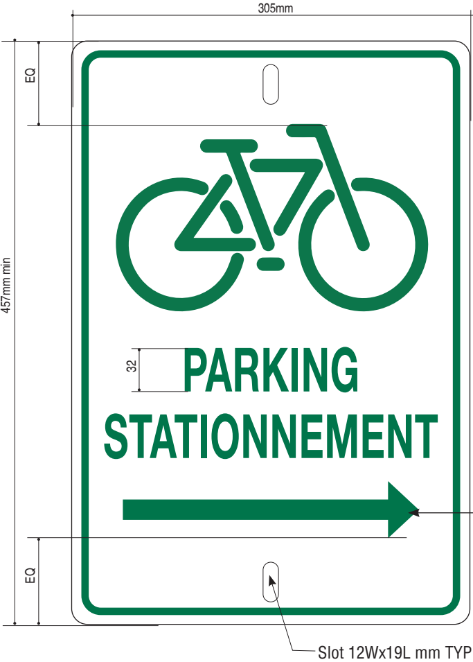
M11.5a Notification Sign - Parking and Traffic-Bike Parking Direction 305mm x 457mm x 3mm Scale 1:4 3mm thick Aluminum with radius corners, with Digital print on reflective applied to face. Sign to be installed to existing surface using appropriate screws and fasteners, 1500 ± 25mm to floor from sign center.
