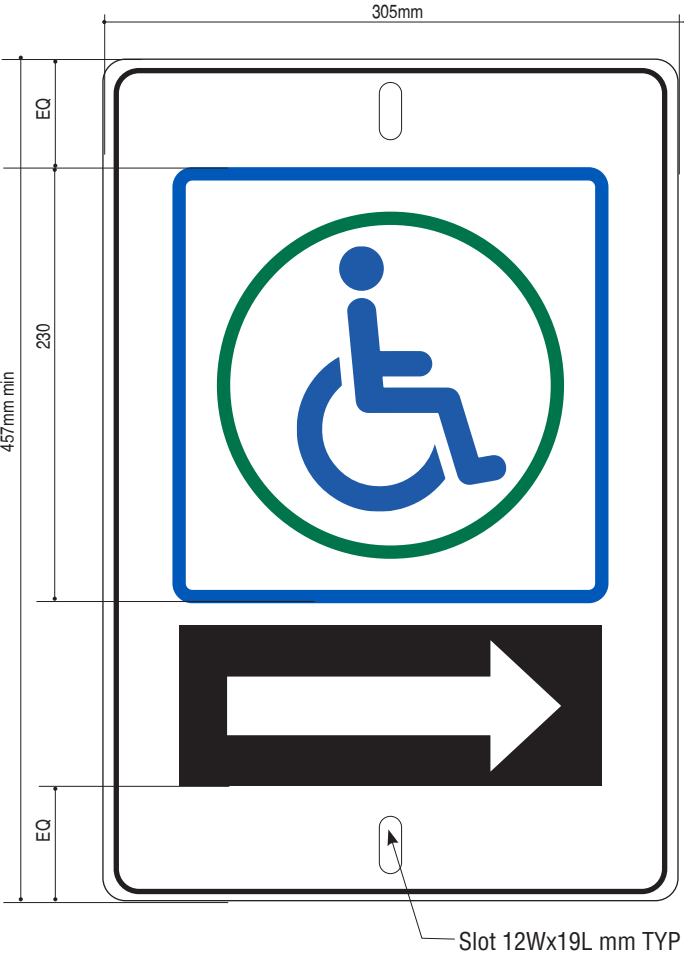
M11.4a Notification Sign - Parking and Traffic-Handicapped Parking Direction 305mm x 457mm x 3mm Scale 1:4 3mm thick Aluminum with radius corners, with Digital print on reflective applied to face. Sign to be installed to existing surface using appropriate screws and fasteners, 1500 ± 25mm to floor from sign center.
