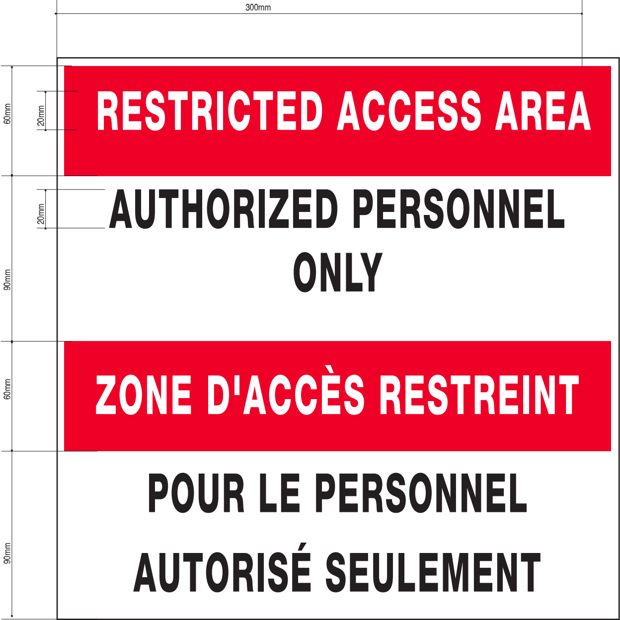
W5-W-162 Warning Sign - Access Area 300mm x 300mm x 3mm Scale 1:2 3mm ACM with direct surface printed graphics. Clear protective laminate. Mounted centered on door 1500 ± 25mm to floor from sign center at all Loading Dock entrance doors (3 signs).
