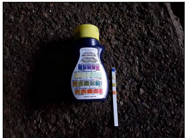
Photo 48 - Water test results: water hardness 0 ppm, total bromine 0 ppm, total alkalinity 40 ppm, and pH of 6.8.
