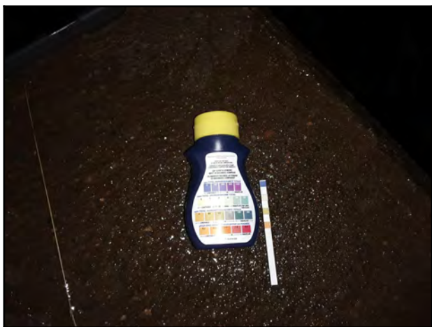
Photo 39 - Water test results: water hardness 0 ppm, total bromine 0 ppm, total alkalinity 0 ppm, and pH of 6.8.
