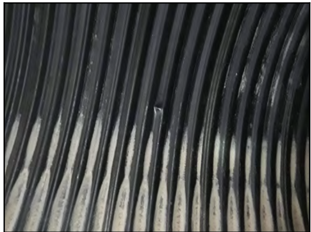
Photo 22 - Small dent near the inlet, measuring approximately 30 mm in depth.
