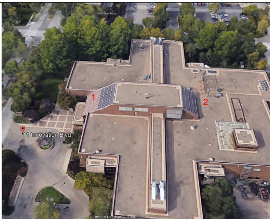
Photo 1 Shows the roof configuration with the first sloped glazing system (Skylight 1) located at the South side; while the second sloped glazing system (Skylight 2) is located at the North side
