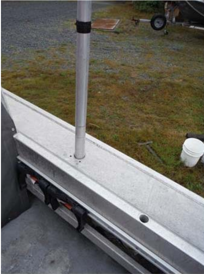
Picture 5: Picture pipe insert that can house a davit or line hauler p
