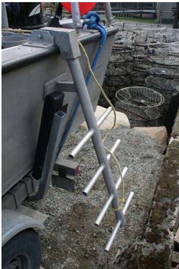
Picture 1: Dive ladder bolt-on bracket design
