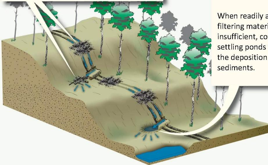
When readily available filtering material is insufficient, construct settling ponds to allow the deposition of sediments.
