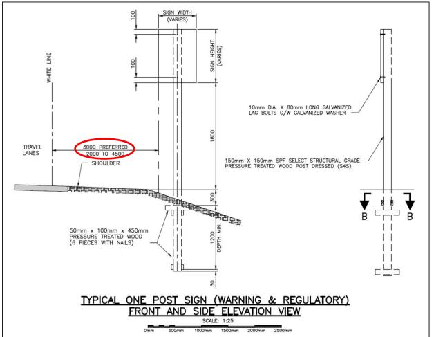
b) For additional drawing G01/G03 "TYPICAL ONE POST SIGN (WARNING & REGULATORY) 2D" Change the dimension circled in red ("3000 preferred") to the following: "DIRECTION OF THE DEPARTMENTAL REPRESENTATIVE"
