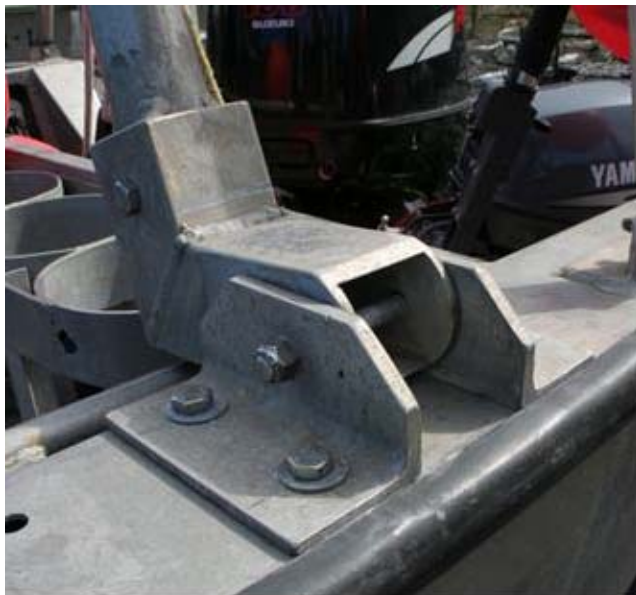
Picture 1: Dive ladder bolt-on bracket design
