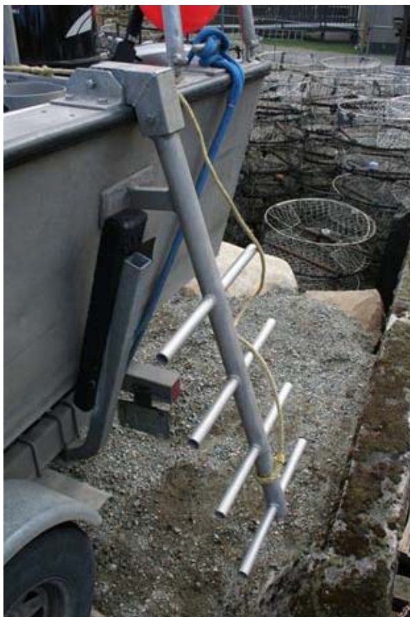
Picture 1: Dive ladder bolt-on bracket design
