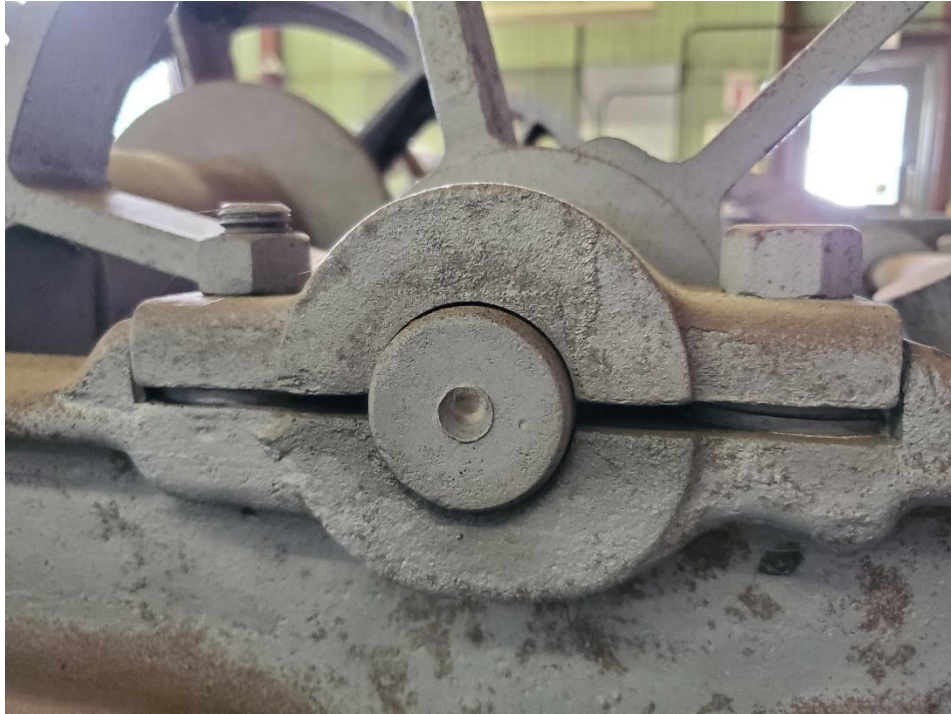
Figure 4.0 – Split pillow block housing with shims installed
