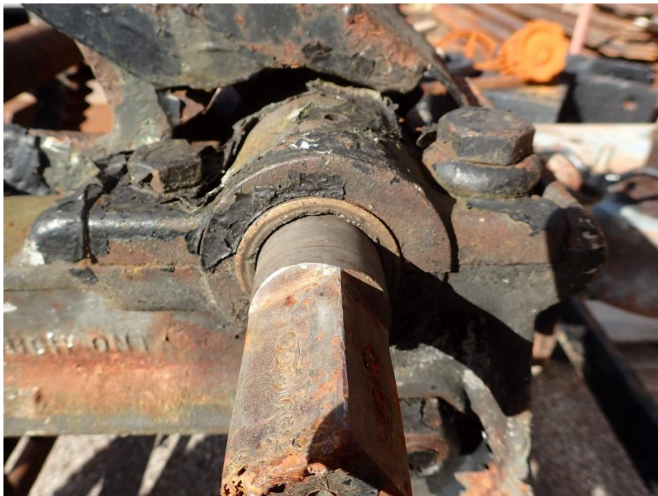
Figure 5.1 – Split pillow block housing with brass bushing
