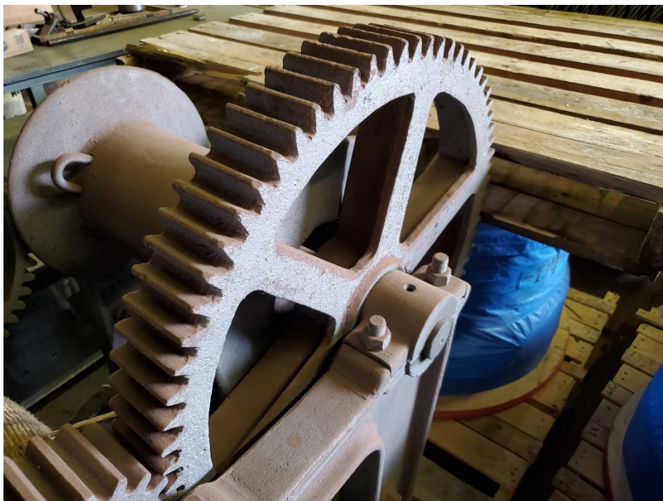
Figure 3.1 – Gearing requiring shielding/guarding
