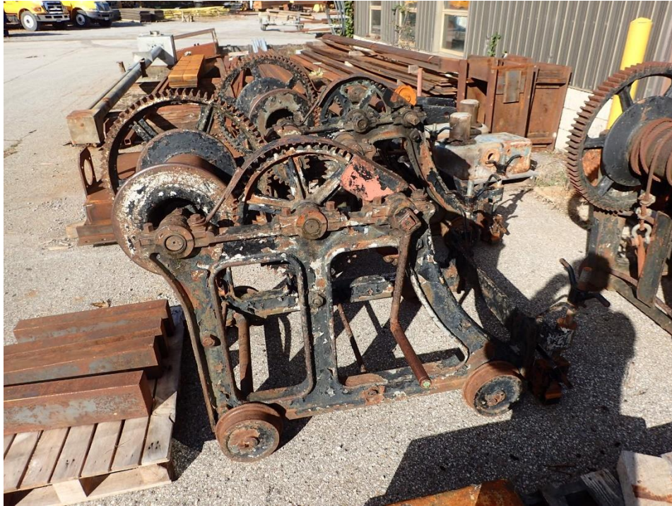
Figure 2.0 – Crab winch typical condition
