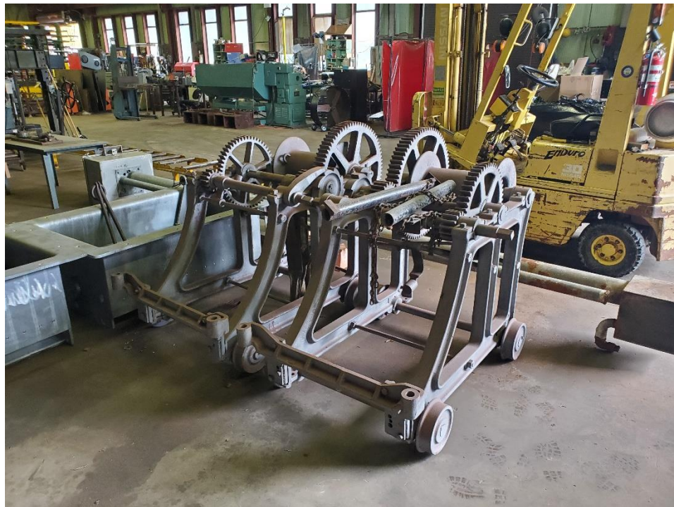
Figure 1.1 – Crab winch set – Sand Blasted
