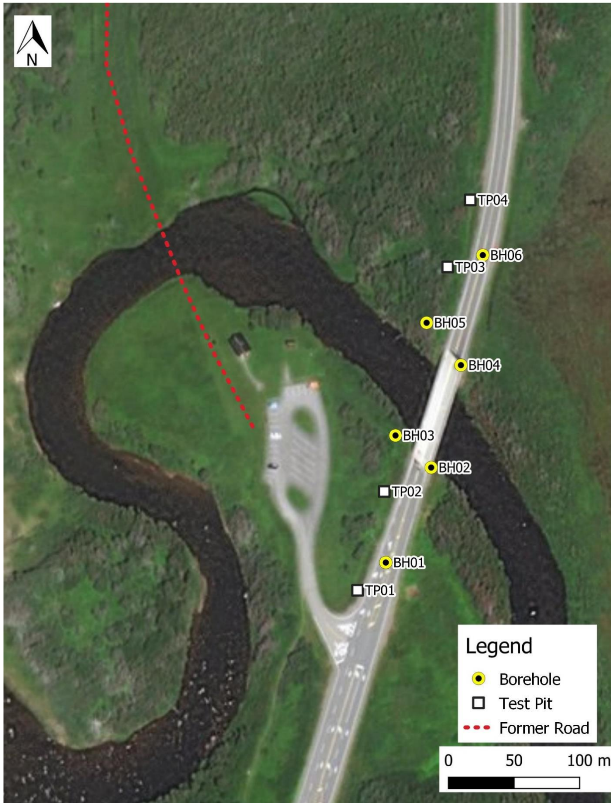
Figure 4: Borehole and test pit locations provided by Harbourside Engineering, as well as location of former road / access road, as indicated in Public Works 1981 Note. Test Pits TP02 and TP03 were not tested following Dec 2019 discussions with Field Unit (Higdon 2019, Harbourside 2020b).
