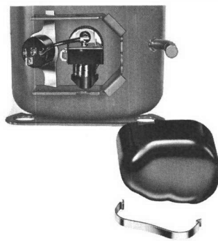
Here the overload and relay are shown assembled in their proper position. Newer relays will have a boss in the center as a stop for the lead to the overload.
