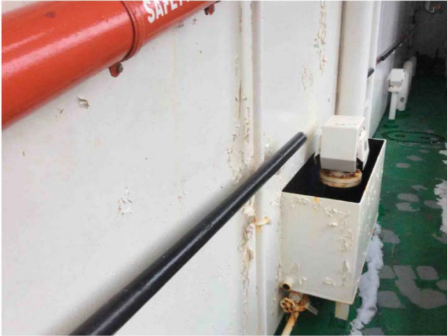
25 Paint sample Outdoor — Wall — White — Poor — Lead-free paint Chantal.Soulard - 2022-02-07 15:55
