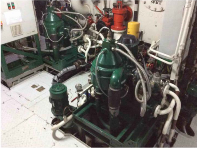
17 Paint sample Engine Room — Equipment — Green — Good — Lead-based paint Chantal.Soulard - 2022-02-07 15:25
