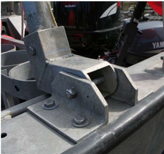
Picture 1: Dive ladder bolt-on bracket design
