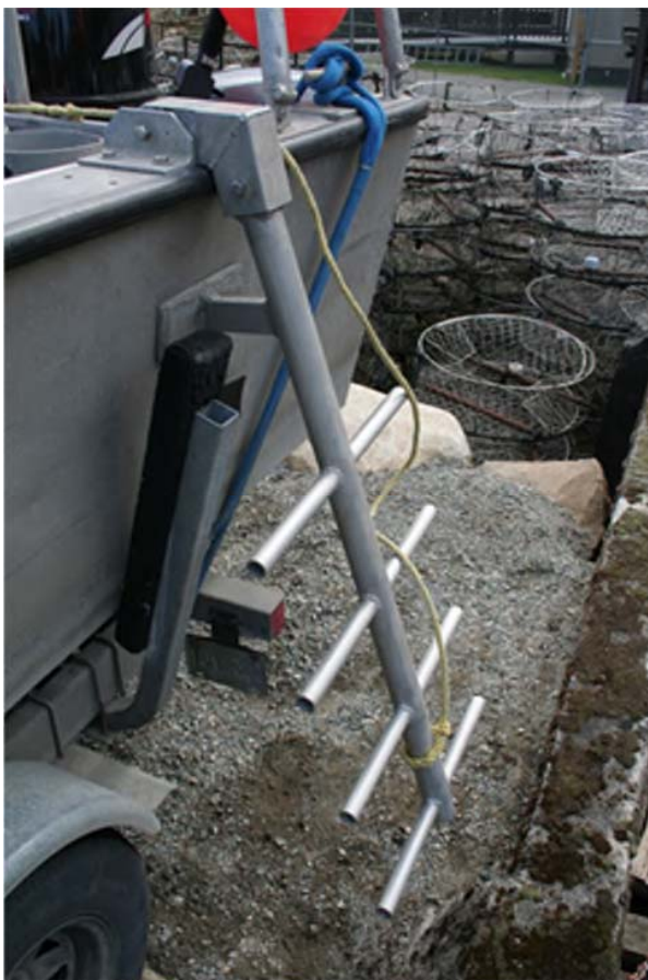
Picture 1: Dive ladder bolt-on bracket design
