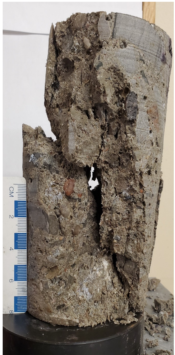
Photo 3B – Core No. 3 Post Compression
