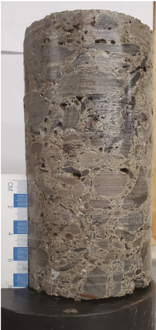
Photo 2A – Core No. 2 Pre-Compression
