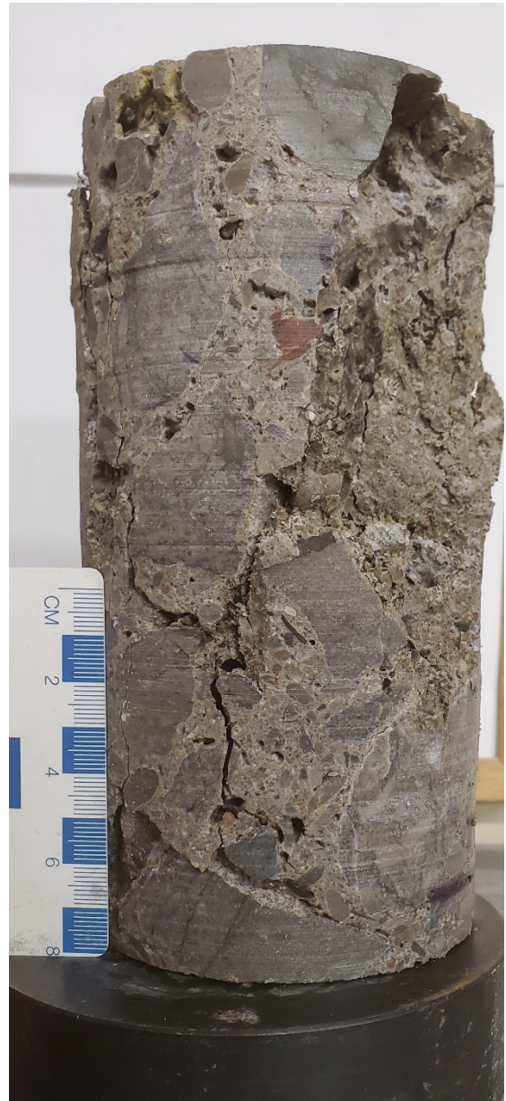
Photo 1B – Core No. 1 Post Compression
