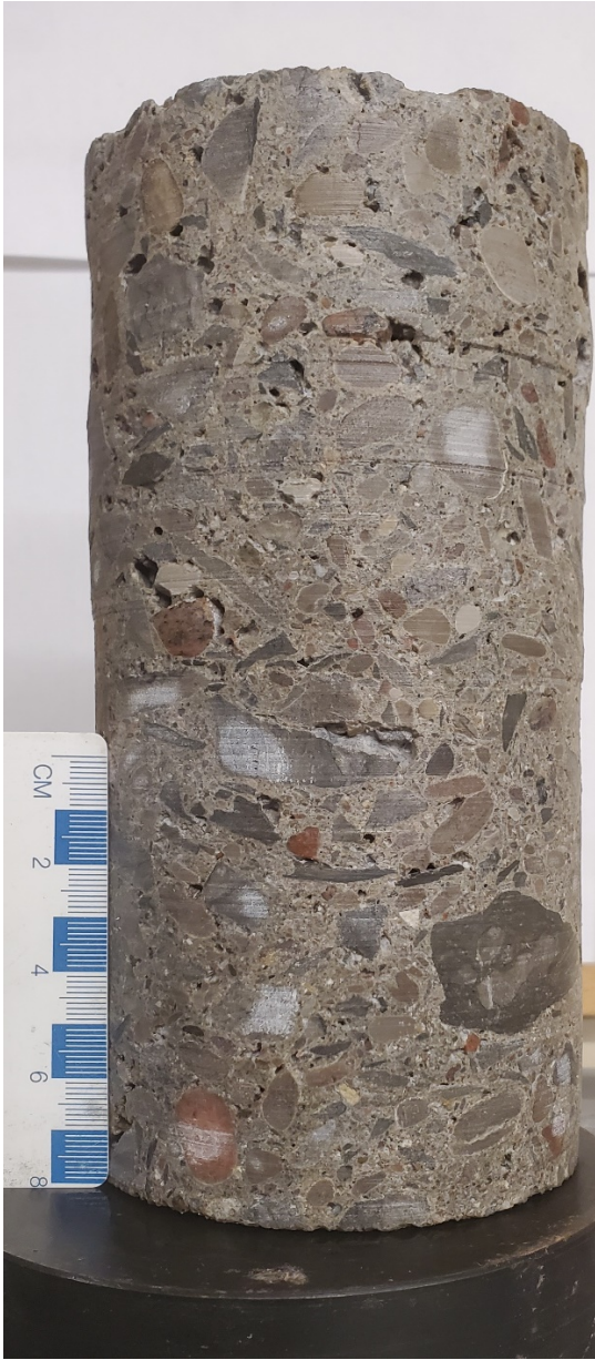
Photo 1A - Core No. 1 Pre-Compression
