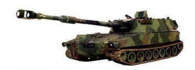
The M109 armoured vehicle is 29.66' (9.04 metres) long; 10.34' (3.15 metres) wide and 10.77' (3.28 metres) high. The weight is 55,049.43 pounds (24,970 kilograms)
