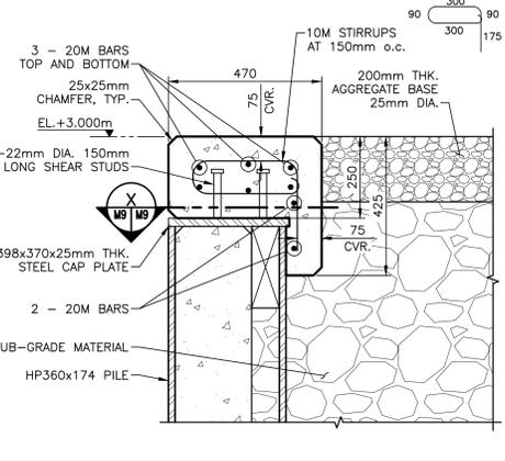
**PILE CAP BEYOND DECK SECTION AT PILE W**
