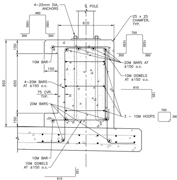
DETAIL - LIGHT POLE PILASTER REINFORCING
