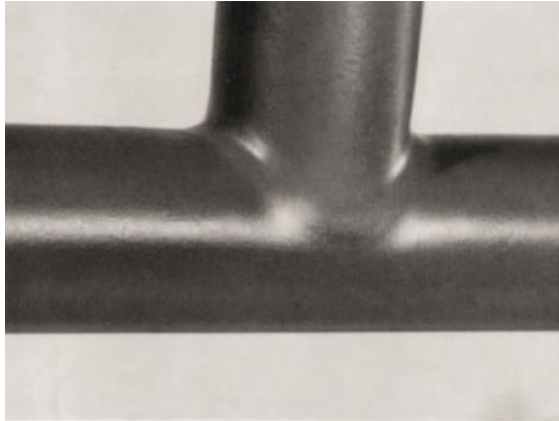
Type 1 Ornamental quality No trace of solder joint.
