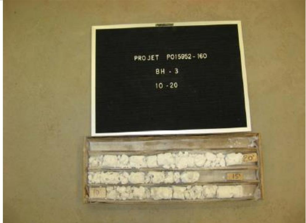
The photograph shows a wooden tray containing three horizontal sections of soil and rock core samples. Above the tray is a black label with white text that reads: "PROJET P015952 - 160", "BH - 3", and "10 - 20". The samples in the tray are light-colored and appear to be soil or soft rock. The tray has small labels "10", "15", and "20" on the right side, corresponding to the depth markers in the description.
