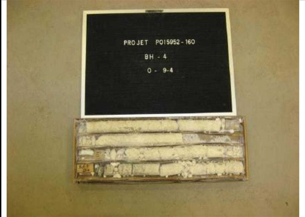
The photograph shows a rectangular wooden tray containing several horizontal sections of soil and rock core samples. Above the tray is a black label with white text that reads: "PROJET PO15952-160", "BH - 4", and "O - 9-4". The samples in the tray appear to be light-colored, possibly sandy or silty soil, with some darker, more crystalline rock fragments interspersed.
