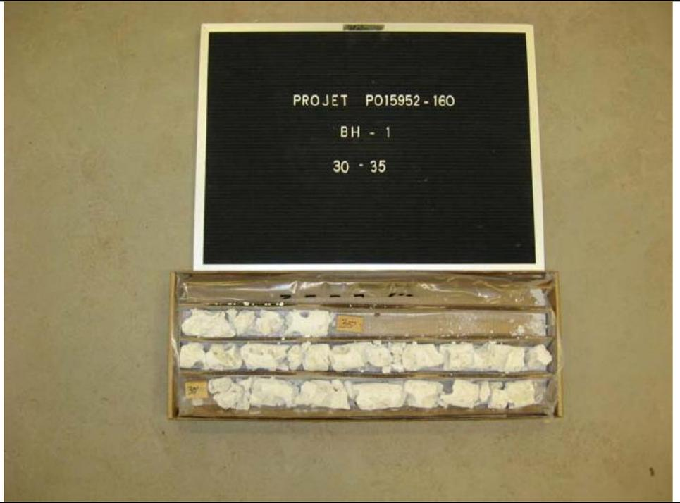
The photograph shows a rectangular box containing three horizontal compartments of soil and rock samples. Above the box is a black label with white text that reads: "PROJET P015952 - 160", "BH - 1", and "30 - 35". The samples appear to be light-colored, possibly silty or sandy soil, with some darker, more fragmented material in the compartments.
