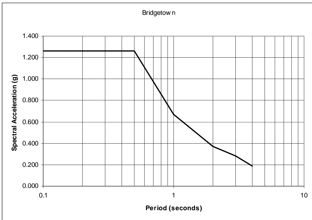
Figure 2: Seismic Hazard Curve Bridgetown, Site Class C
