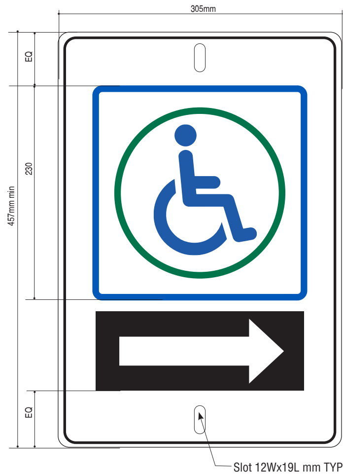
M11.4a Notification Sign - Parking and Traffic-Handicapped Parking Direction 305mm x 457mm x 3mm Scale 1:4 3mm thick Aluminum with radius corners, with Digital print on reflective applied to face. Sign to be installed to existing surface using appropriate screws and fasteners, 1500 ± 25mm to floor from sign center.
