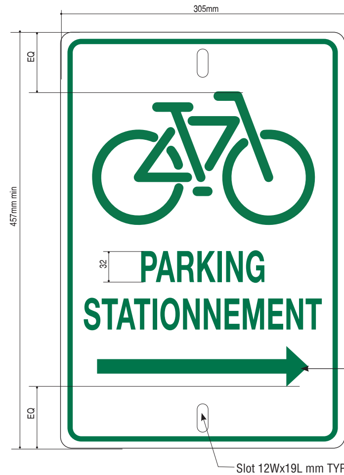
M11.5a Notification Sign - Parking and Traffic-Bike Parking Direction 305mm x 457mm x 3mm Scale 1:4 3mm thick Aluminum with radius corners, with Digital print on reflective applied to face. Sign to be installed to existing surface using appropriate screws and fasteners, 1500 ± 25mm to floor from sign center.
