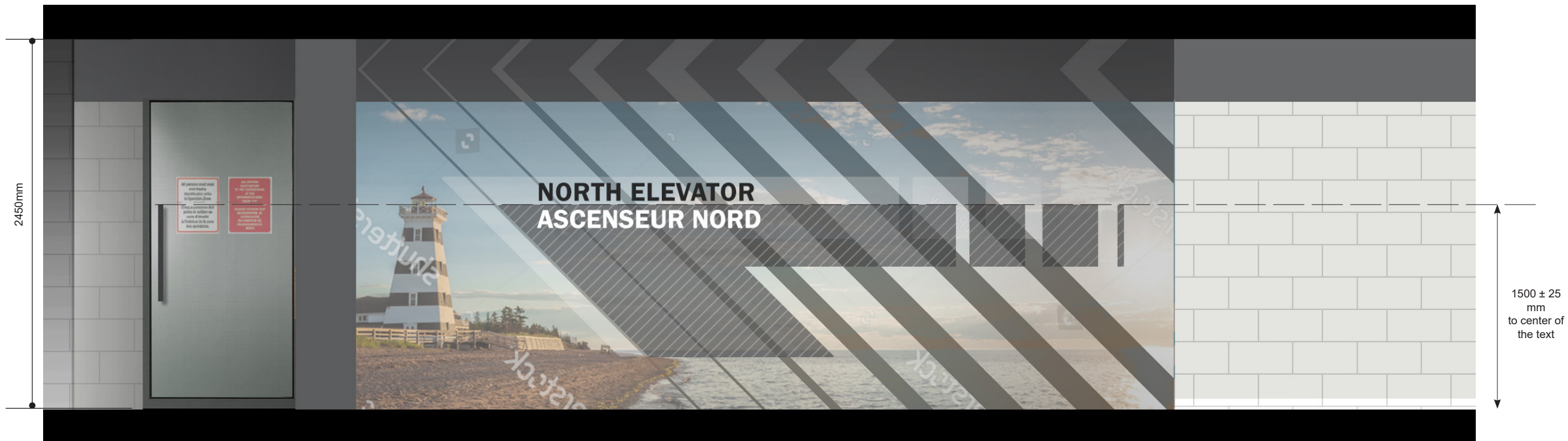
Detail N.T.S. Wall-mounted Acrylic Digital Printed Film over concrete blocks, Opaque.
