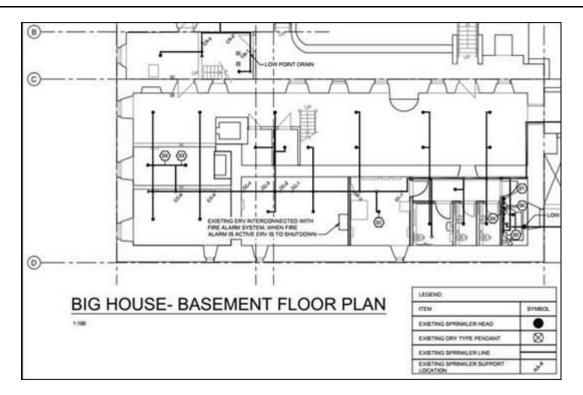
**Q19** Drawing M1.2...Note 01 – Install new dry type pendant. The piping to this particular sprinkler head appears to be removed. It also appears as though a low point drain may have to be added to accommodate the slope. Can you confirm that we are to reinstall the piping and that we may install a new low point drain?
