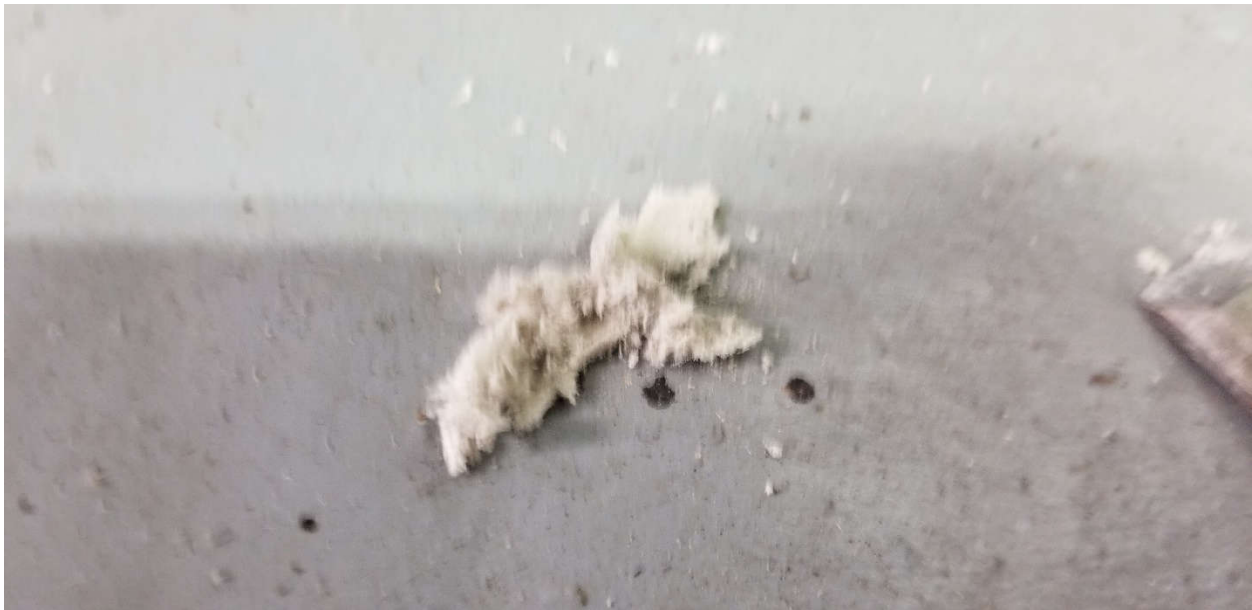
Photograph 4: Grey fibrous wall coating, collected from the Penthouse perimeter wall, contains 35% Chrysotile asbestos (Sample ID 41133-16A).
