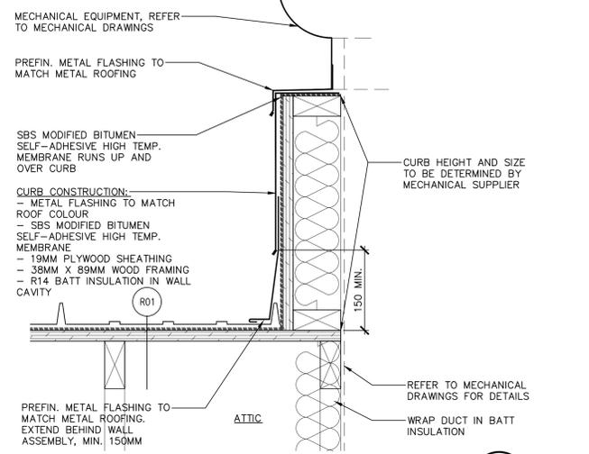
SECTION DETAIL: ROOF CURB
