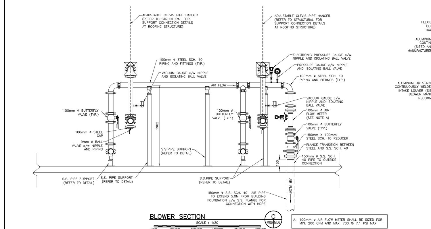
A. 100mm Ø AIR FLOW METER SHALL BE SIZED FOR MIN. 200 CFM AND MAX. 700 @ 7.1 PSI MAX.
