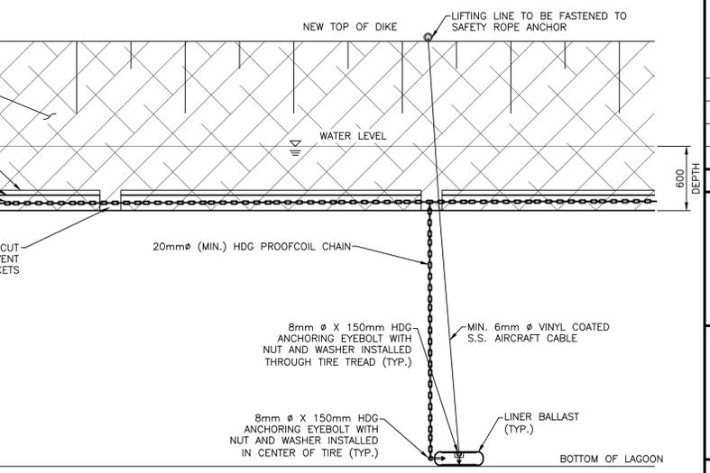
DETAIL - CELL #1 AESTHETIC LINER ANCHORING & LOCKING TRENCH
