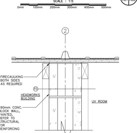
SECTION DETAIL: P3 WALL AT ROOF
