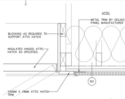
SECTION DETAIL: ATTIC HATCH
