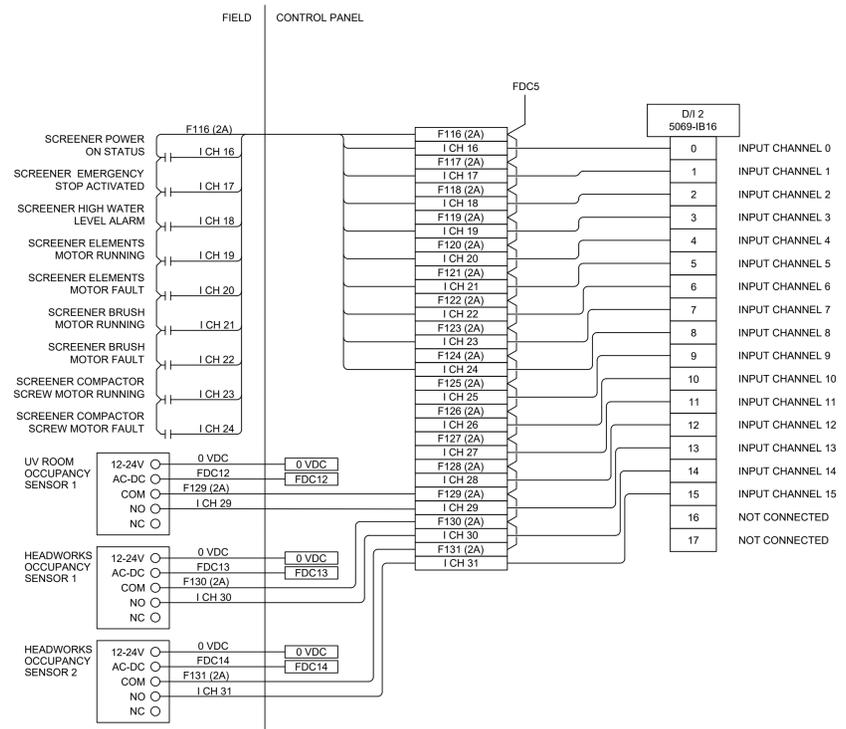
RACK 1 SLOT 5 DISCRETE DC INPUT CARD 2
