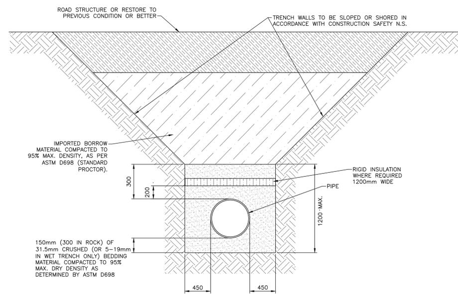
DETAIL - TYPICAL PIPE TRENCH SECTION
