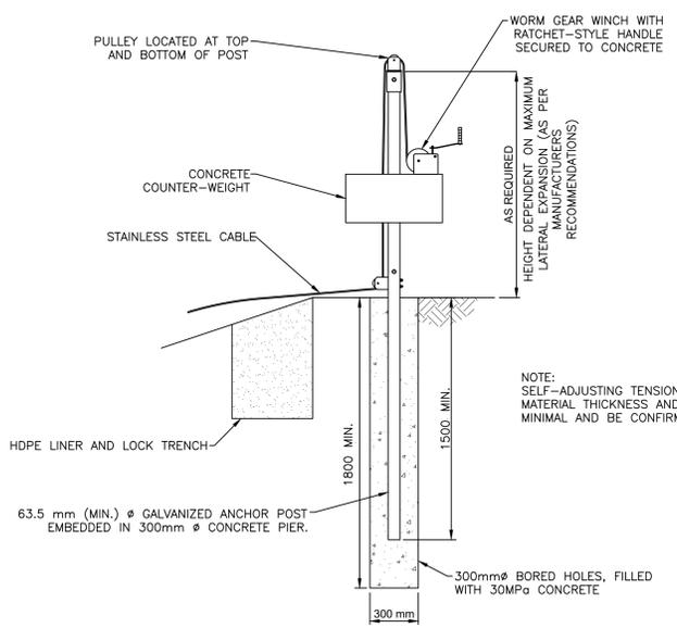
SELF-ADJUSTING TENSION ASSEMBLY (AT LATERAL FREE END) N.T.S.
