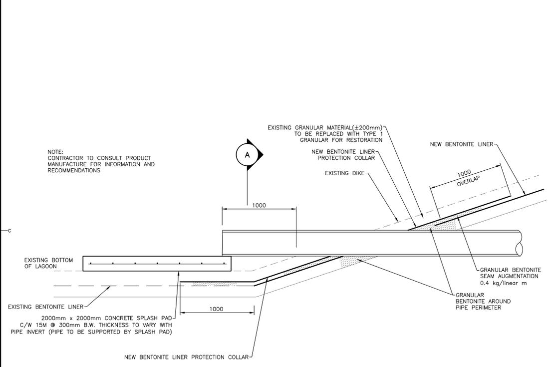
DETAIL - PIPE PENETRATION THRU EXISTING CELL #01 & SPLASH PAD
