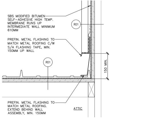
SECTION DETAIL: ROOF INTERMEDIATE WALL
