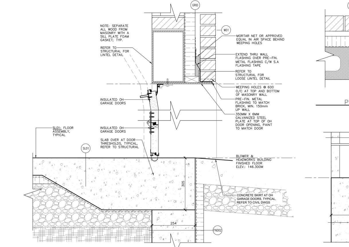
SECTION DETAIL: O/H DOOR HEAD/ SILL
