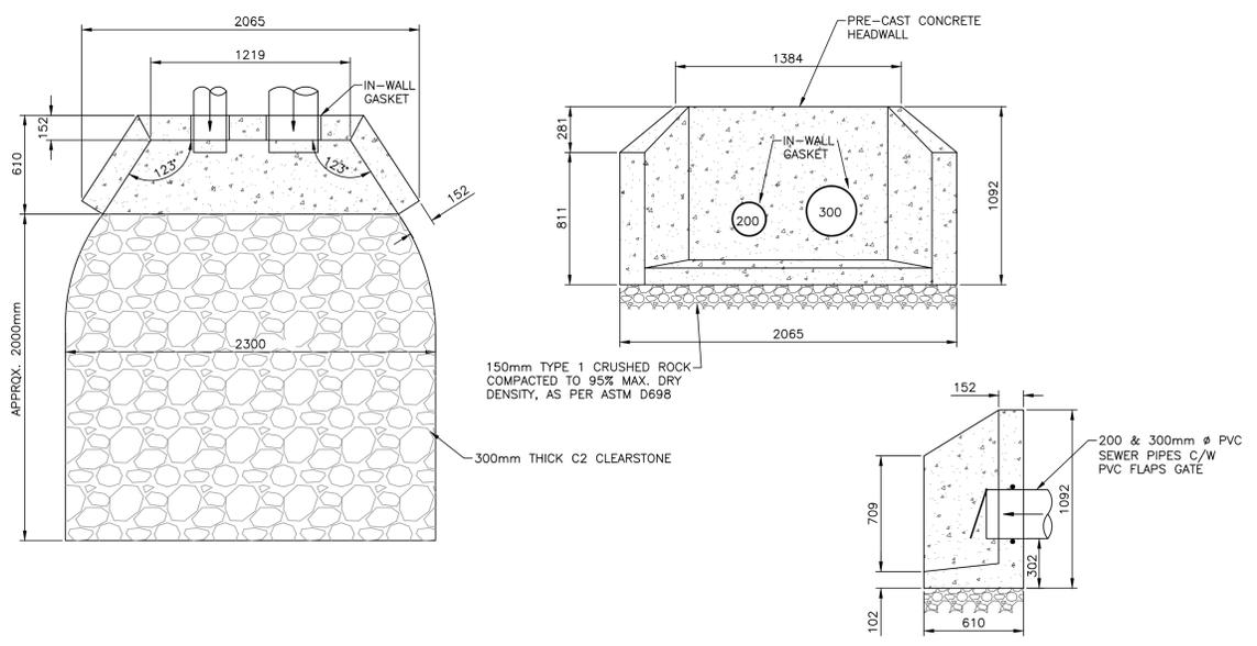
PRECAST CONCRETE HEADWALL DETAIL
