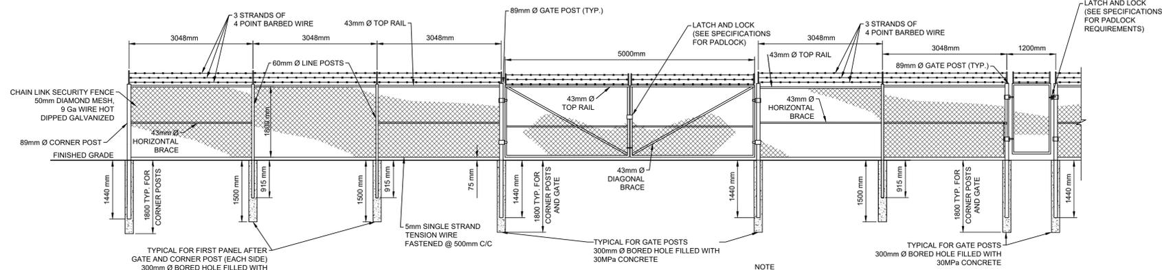
DETAIL - CHAIN LINK FENCE C/W DOUBLE VEHICLE GATE
