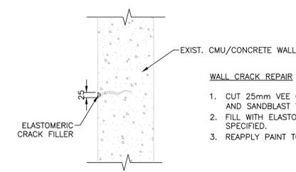
**1 WALL CRACK REPAIR - SECTION**
