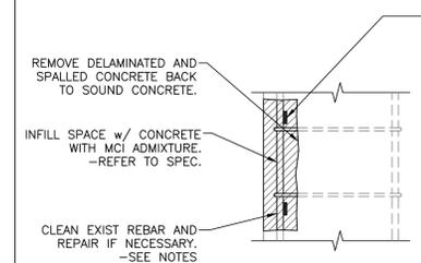
**4B COLUMN REPAIR - ELEVATION**
