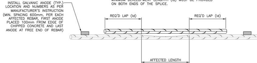
1 S01 TYPICAL REBAR REPAIR (LAP SPlice)
