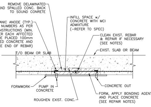
**3A SOFFIT DEEP SPALLING - DETAIL**
