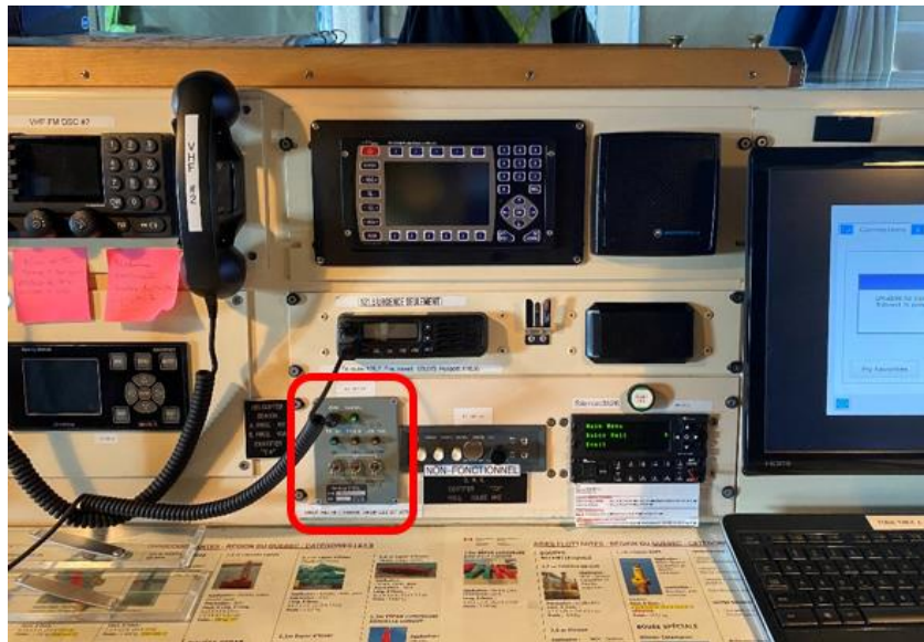
Figure 18.8-3: NDB Remote Control Unit
