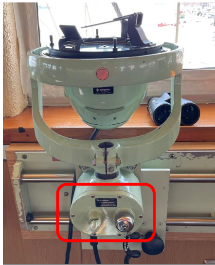
Figure 18.2-7: Cover plate to be replaced
