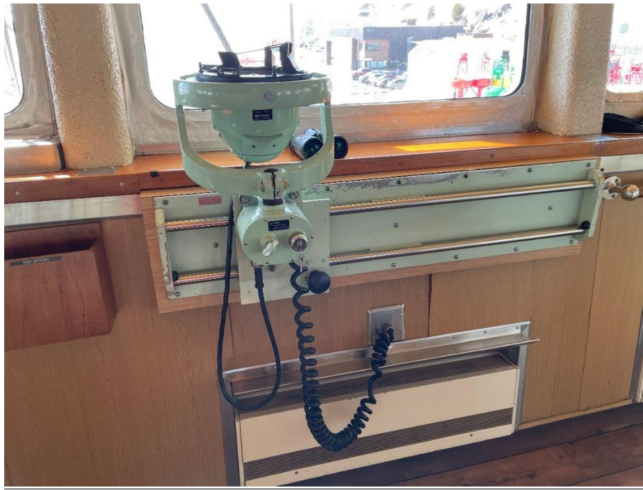
Figure 18.2-8: Bearing repeater on sliding rail (Fwd centre)
