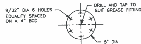
SHAFT SLEEVE COVER DETAIL
