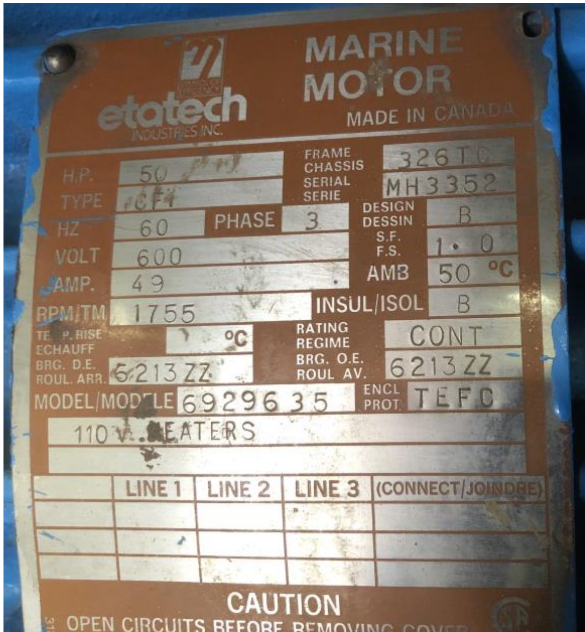
Nameplate of the Pump motor
