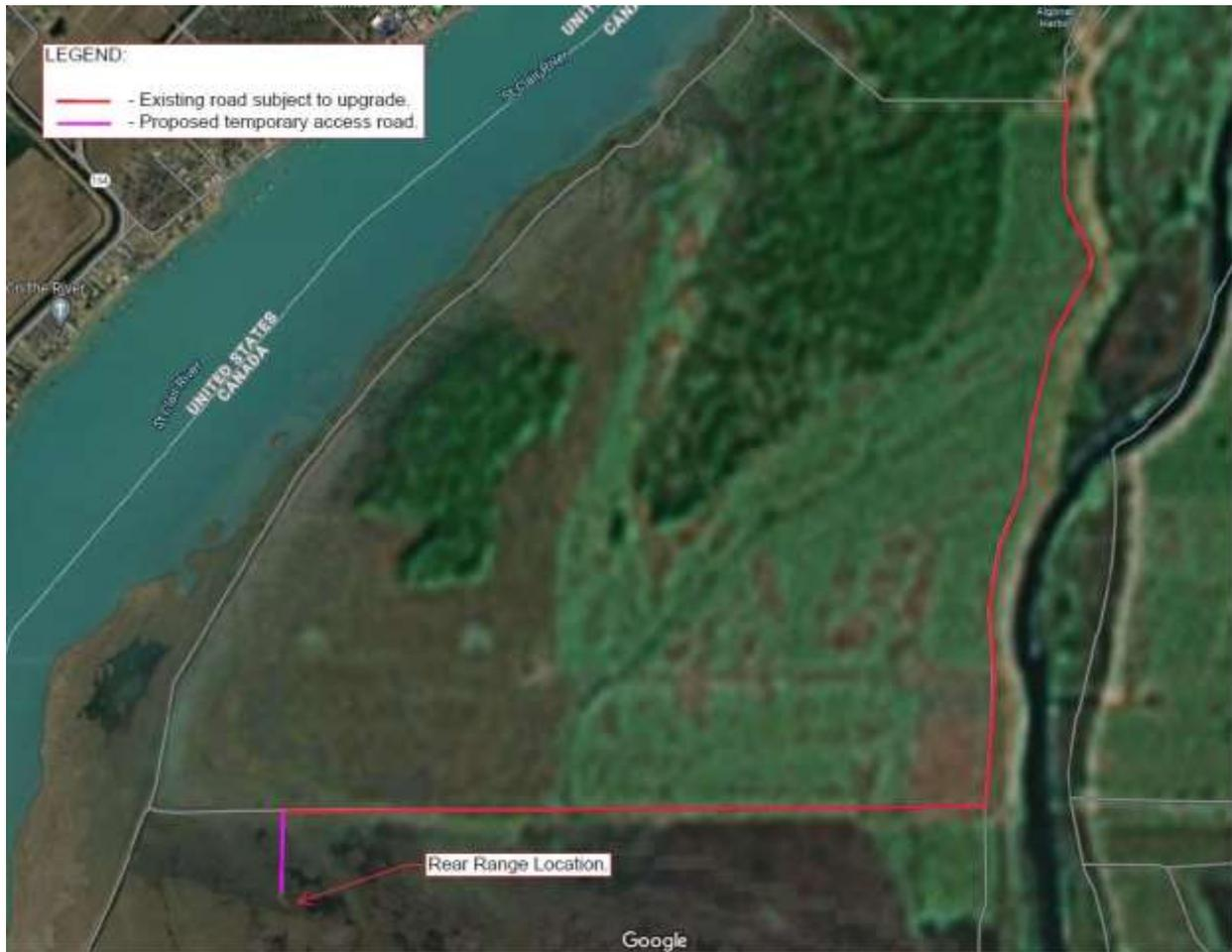
Figure 6 – Extents of existing road subject to road upgrade and location of proposed temporary access road.
