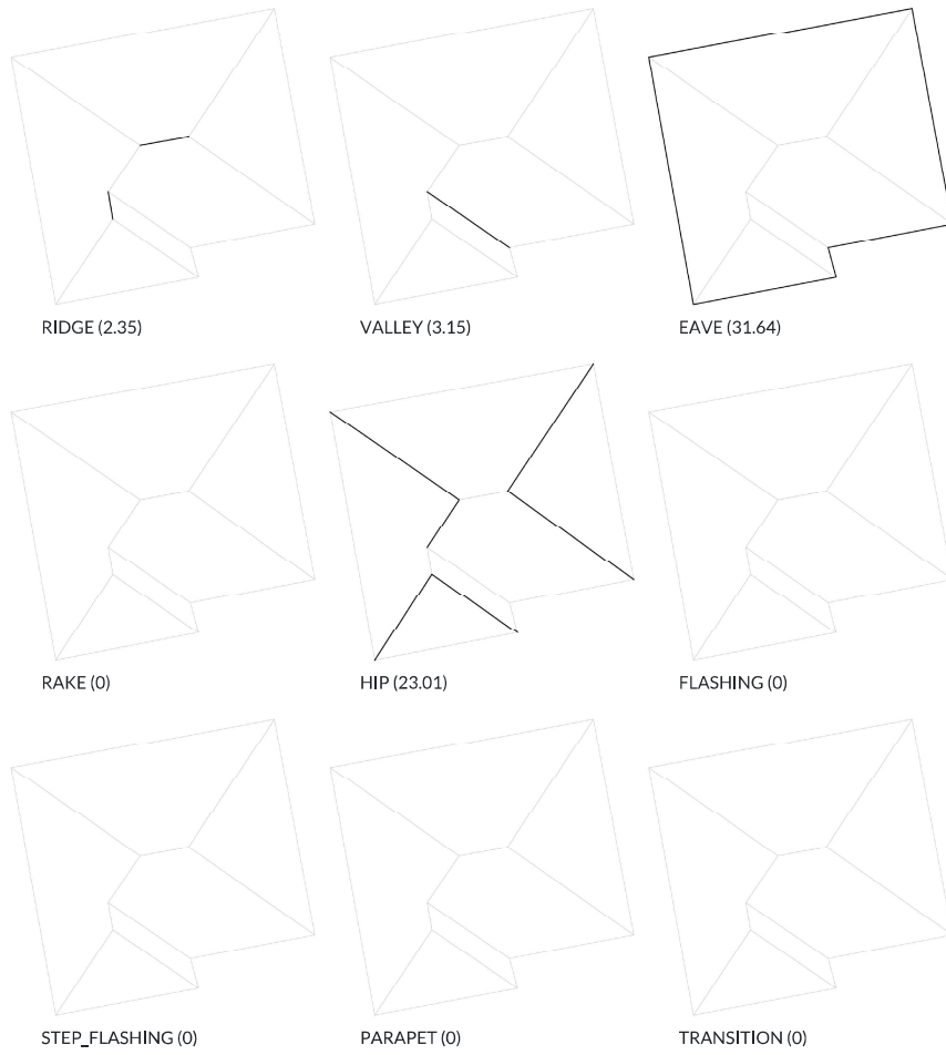
Figure 5: Roof Edge Classification (units: meters)
