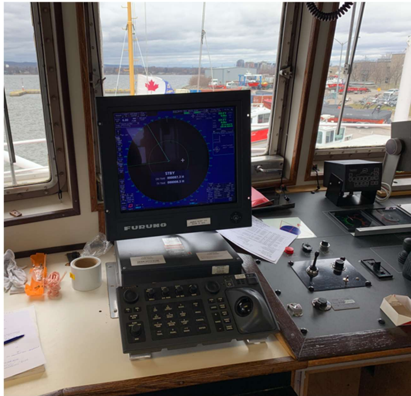
Figure 18.2.D – PORT Radar Processor & Display Location
