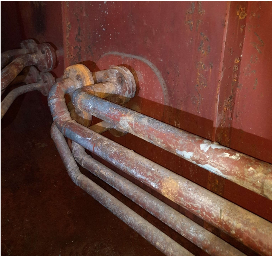
Figure 15.5.D – PW lines, transits thru bulkhead at frame 32
