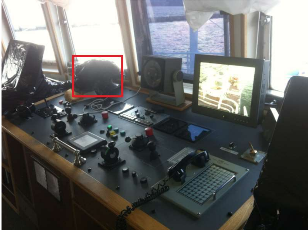
Figure 18.1.E – Control and Display Unit Installation Location
