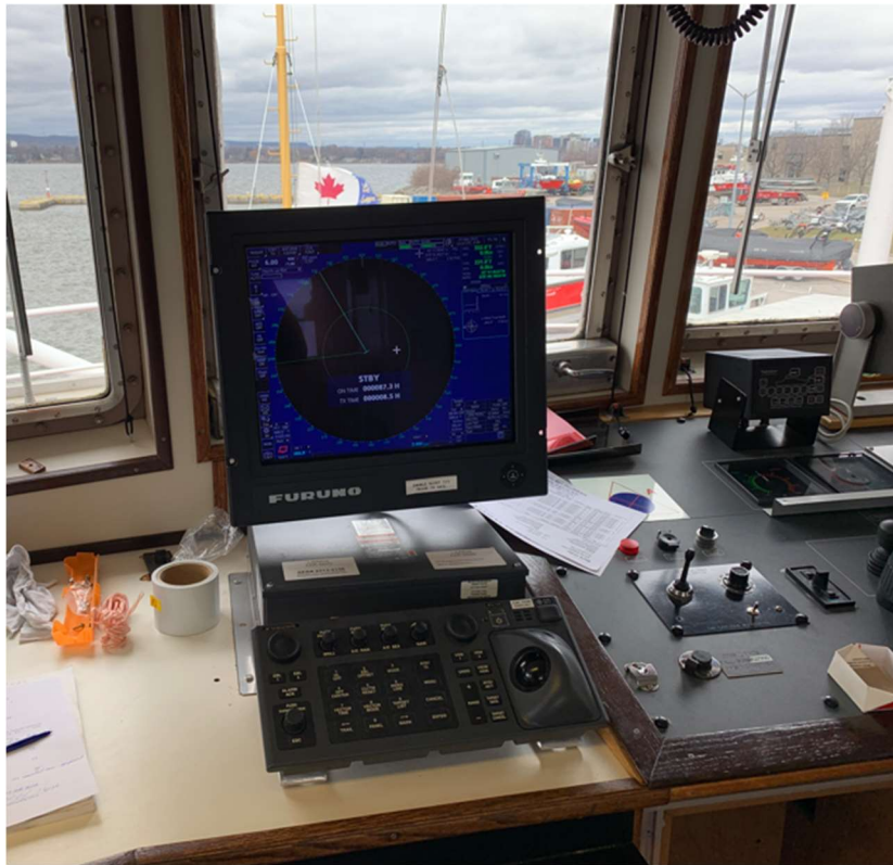
Figure 18.2.D – PORT Radar Processor & Display Location
