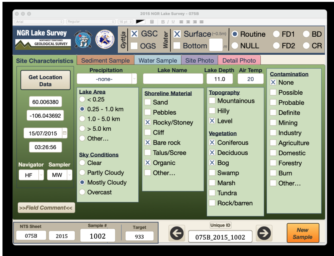
Figure 1. The first tab of the digital field card includes fields for recording location and general environmental conditions.
