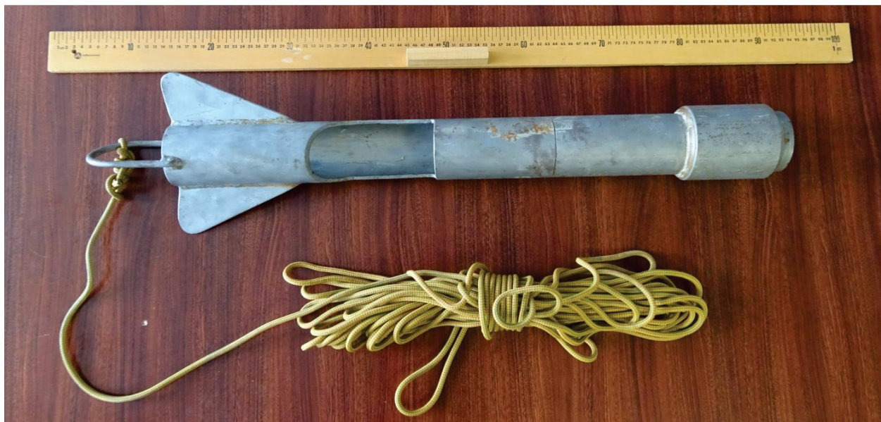
Figure 2. Lake sediment sampler used at the Geological Survey of Canada. The device weighs 7.1 kg and collects a 30 cm core sample of lake sediment, corresponding to a weight of 1.2 kg of lake sediment.
