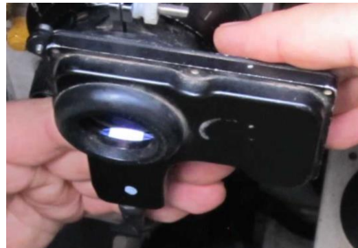
Tracer Burst Unit (simulates fall of shot, gives feedback to gunner)
