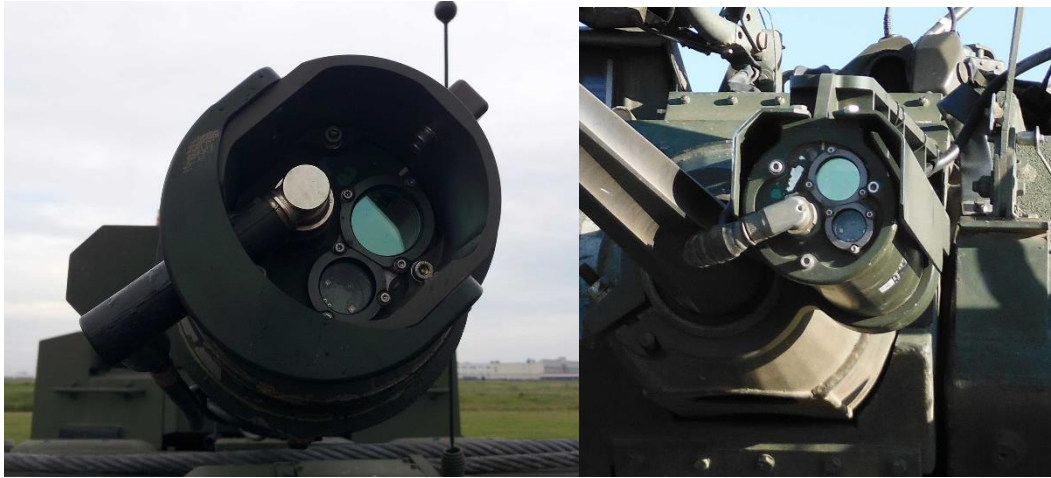
Laser Transmitter Unit Mounted in 120mm cannon (left) Mounted by 25mm cannon (right)
