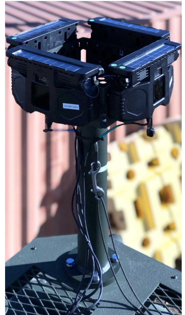
Mast with four High Sensitivity Detectors and built in lights
