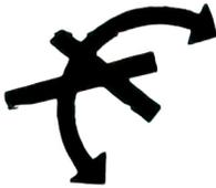
TO INDICATE THAT THE SHIPPING CONTAINER SHALL NOT BE ROLLED.
