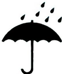
TO INDICATE THAT THE SHIPPING CONTAINER SHALL BE KEPT IN A DRY ENVIRONMENT.
