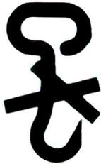
TO INDICATE THAT HOOKS ARE PROHIBITED FOR LIFTING THE SHIPPING CONTAINER.
