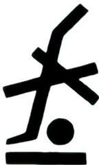
TO INDICATE WHERE HAND TRUCKS OR DOLLIES SHALL NOT BE PLACED WHEN HANDLING THE SHIPPING CONTAINER.
