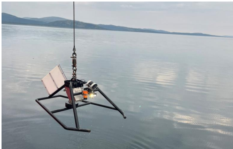
Figure 3. Drop camera platform attachment. Weight is roughly 500lbs.
