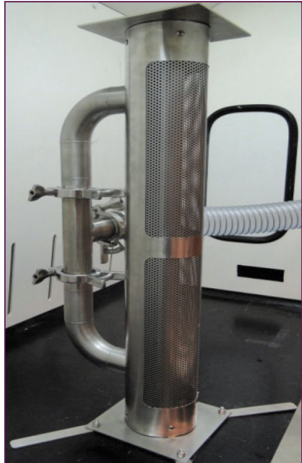
Figure A-4: Smoke Diffuser
