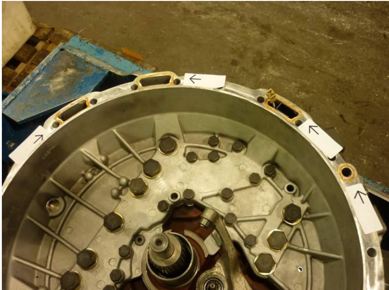
Figure 1: Clutch housing and mating housing (not shown) – Application of Loctite 574 Flange Sealant
