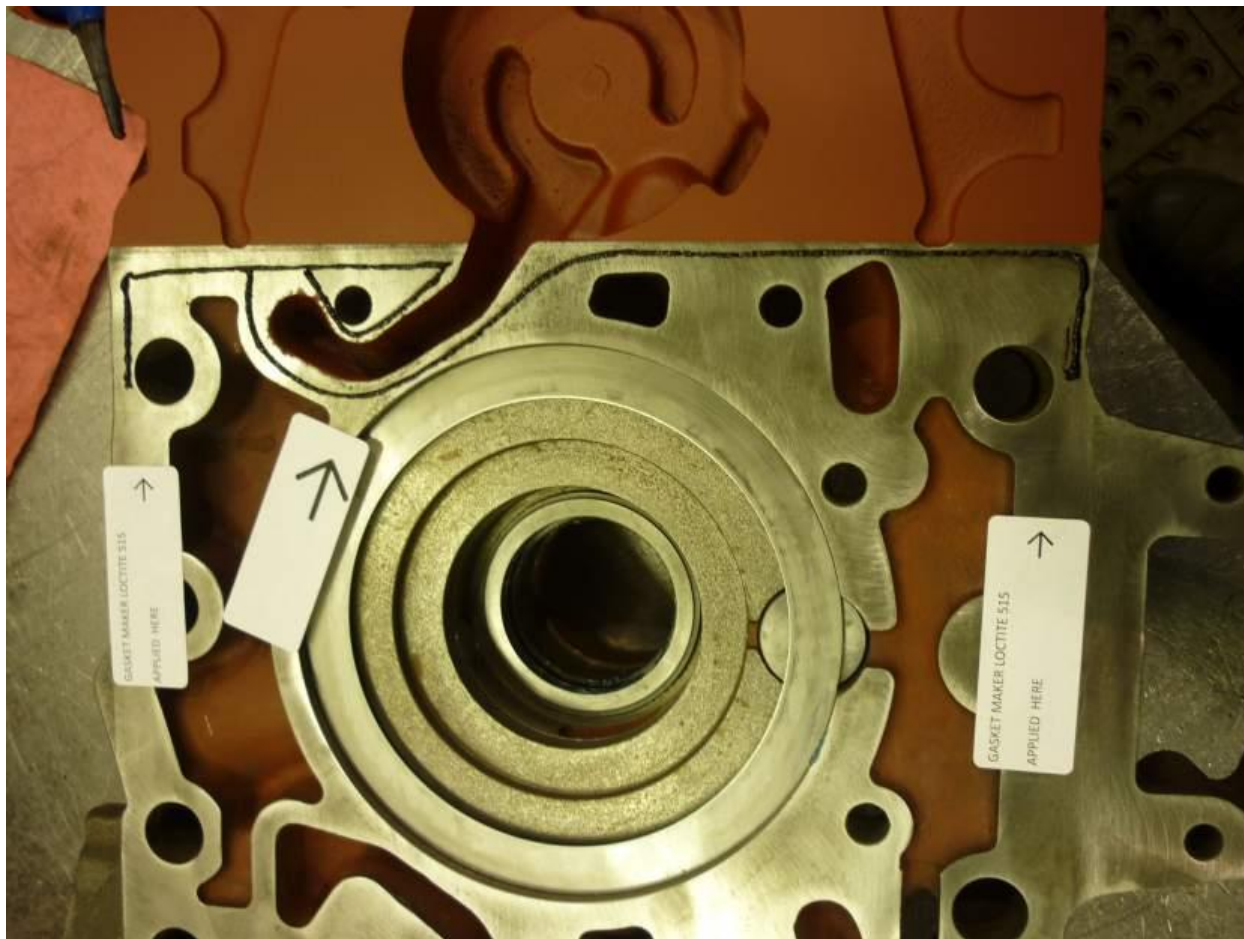
Figure 3: Connecting housing – Application of Loctite 515 Flange Sealant
