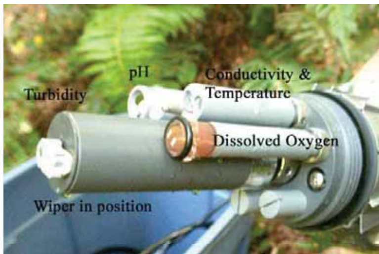
Figure D-9. Examples of some probes used in one kind of sonde. Photo: Judith Burke
