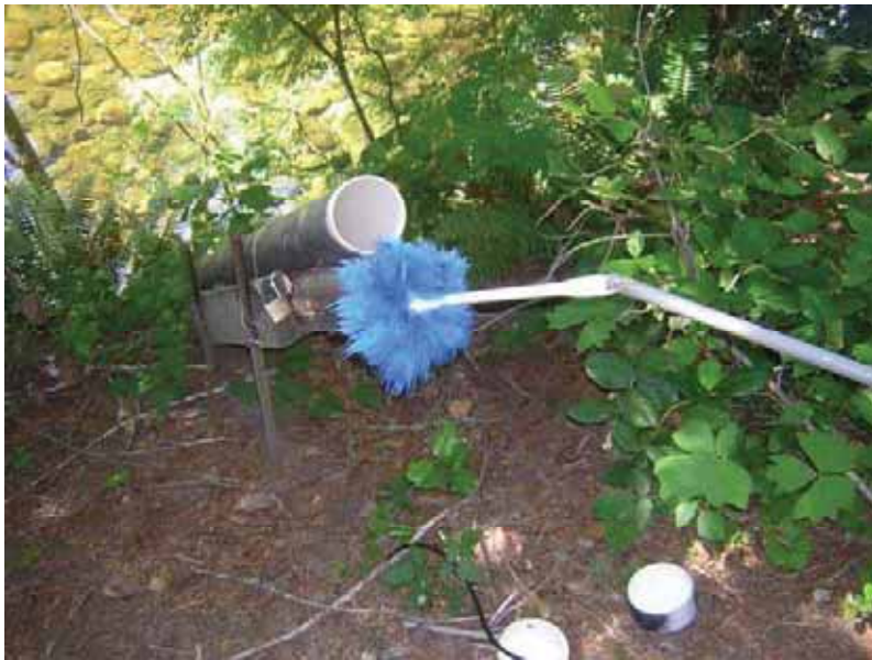
Figure D-7. A mop is used to clean the deployment tube. The tube being cleaned is the one housing the deployed sonde. Photo: George Butcher
