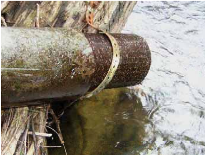
Figure E-2. A poorly designed deployment tube. The section of the tube that covers the guard of the sonde is a heavy metal with slots that are easily clogged with debris, preventing a good flow of water across the tube. Photo: George Butcher.
