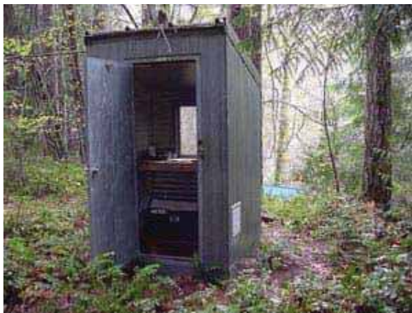
Figure C-2. A walk-in enclosure is one way to protect the equipment. Photo: Judith Burke
