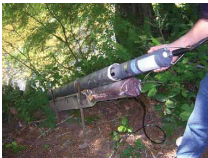
Figure D-18. Deploy the portable sonde in its own deployment tube. Photo: George Butcher
