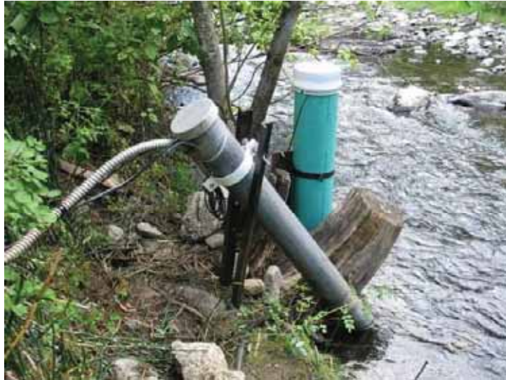
Figure C-4 Deployment tube in Beaver Creek. Note the cable in the casing and the location of the deployment tube on the downstream side of the stump where there is some pooling of water. The vertical tube is a pressure transducer used to measure water level. Photo: Julia Beatty
