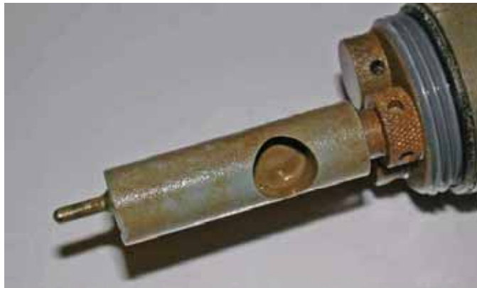
Figure D-8. A conductivity / temperature sensor before cleaning. Note the cleaned conductivity / temperature probe in Figure D-9. Photo: Linda Gregory
