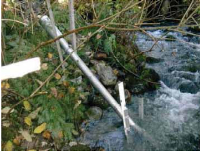
Figure C-5. A metal deployment tube may be required in high velocity and high debris flow conditions. Photo: Rod Shead
