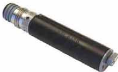
Figure D-15. A turbidity probe with a wiper in the correct position. Photo: Hoskin Scientific
