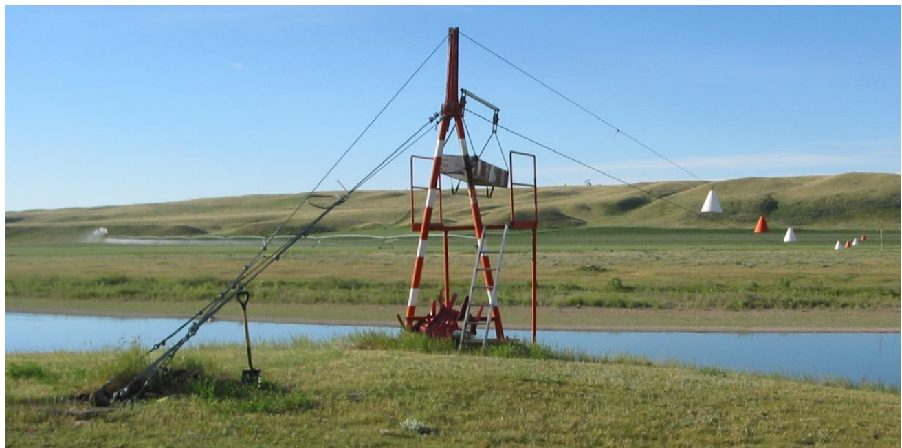
Figure 4. Concrete anchor on left bank home side
