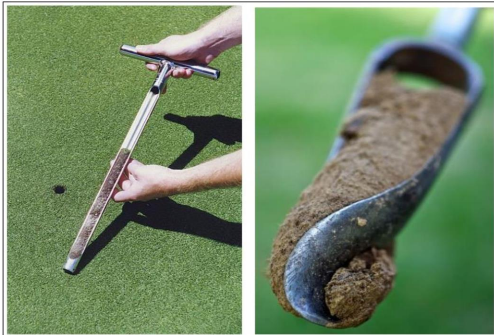
Photograph 1. Left: hand piston sampler. Right: Hand auger sampler.
