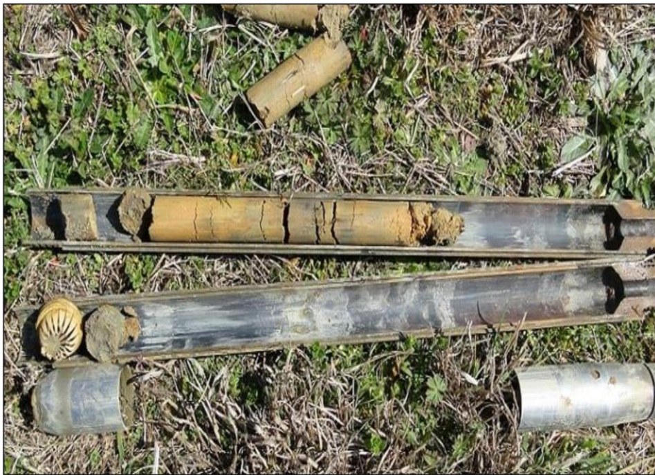
Photograph 3. Drill mounted split spoon sampler.
