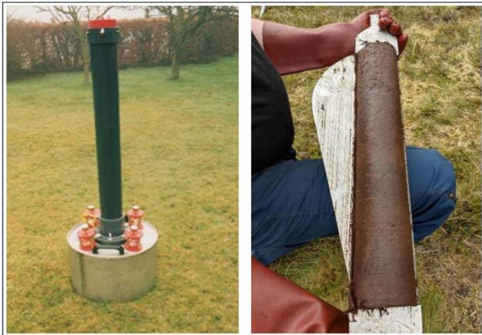
Photograph 2. Left: Submersible Mackereth Corer. Right: Submersible Russian peat corer.
